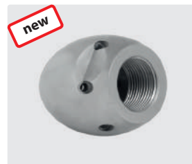
3/4" F. 6x 75° +1x 0°. 30-100 l/min. For (R) Ø 120-250 mm. Outside Ø 50 mm. Ⓢ 567 g.
