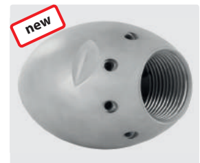
1" F. 8x 75° +1x 0°. 100-250 l/min. For (R) Ø 150-300 mm. Outside Ø 62 mm. Ⓢ 1,265 g.
