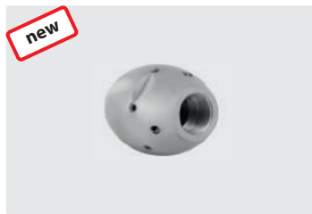
1/4" F. 6x 75° 3x 30° +1x 0°. 25-70 l/min. For (R) Ø 75-150 mm. Outside Ø 30 mm. Ⓢ 223 g.
