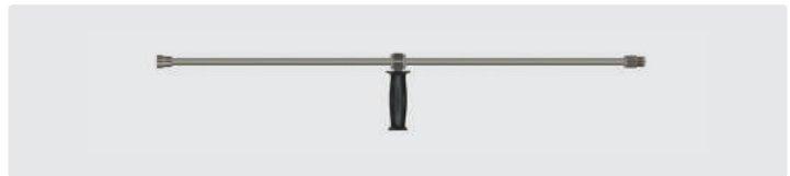
1/2" M. Lance with grip and sleeve 1/4" F NPT stainless steel without high pressure nozzle. Max. 600 bar / 150 °C
