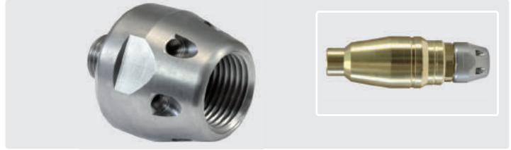
For ST-458/ST-559 rotating nozzles. Hardened stainless steel. Max. 500 bar. \ominus 1/4" M and 6 M5 threads for nozzle inserts (see table below).
