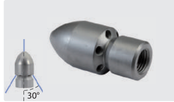
1/4" F. Outside \varnothing 25 mm. 6 rear jets, with front jet
