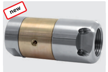
3/4" F. 6 rear jets. 3 side jets. Outside \varnothing 38 mm. ☒ 550 g.
