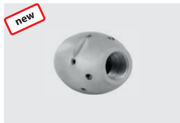
3/8" F. 6x 75° 3x 30° +1x 0°. 30-100 l/min. For (R) Ø 100-200 mm. Outside Ø 35 mm. Ⓢ 314 g.
