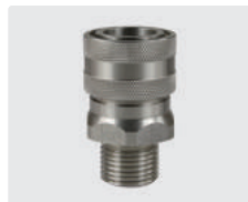
Coupling : M. Stainless steel. 60° cone. Max. 250 bar / 150 °C
