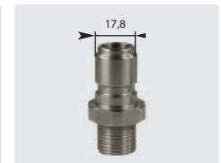
Plug : M. Stainless steel. 60° cone. Max. 250 bar / 150 °C
