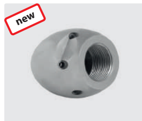
1/2" F. 6x 75° +1x 0°. 30-100 l/min. For (R) Ø 100-200 mm. Outside Ø 40 mm. Ⓢ 281 g.
