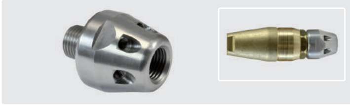
For ST-357/ST-456 rotating nozzles. Hardened stainless steel. Max. 350 bar. \ominus 1/4" M and 6 M5 threads for nozzle inserts (see table below).
