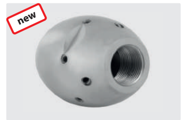
3/4" F. 6x 75° 3x 30° +1x 0°. 100-250 l/min. For (R) Ø 150-300 mm. Outside Ø 50 mm. Ⓢ 1,367 g.
