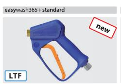
Professional gun. Standard. With swivel running in ball bearing. Max. 310 bar / 45 l/min / 150 °C
